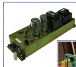
Hand-Crafted All-Tube Amplifier Used on Model 122A, 122XB and 147A Leslies
